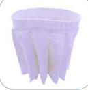
The filtration is guaranteed by a M polyester class filter. The star shape permits the passage of the air also when the filter is dirty. The textile of the filter is in M Class (BIA | En 60335-2-69). It means that all particles till 1 micron are stopped by the filter so as to protect the motors and the operator around the vacuum cleaner.
