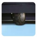
Traction is provided by the rear-drive wheel which ensures great manoeuvrability and safe driving with a very tight turning angle
