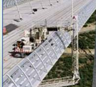
The use of the ABC machines is made possible as well on bridges having very high wind/noise barriers up to 5.4 m. for the standard machines, which can be increased at even bigger height on special request.
