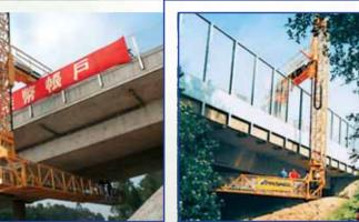
The smallest unit ABC 60 of the range, being mounted on a truckchassis of 3.5 t. GVW only, is specifically designed to enable quick and easy access to the underside of bridges of limited dimensions. Thanks to its high versatility and
