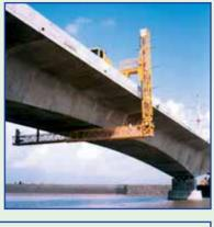
Ideal for rapid inspections as well as for repair works of any kind, the ABC platforms can be supplied with "Assistant Ladder" on board, to enable access of personnel in between girder intradosses.
