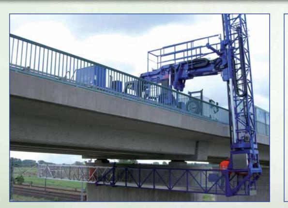
The spacious platforms of the ABC range of machines enable the operators to carry out any sort of heavy-duty repair work underneath bridge decks, by the use of electric/hydraulic/pneumatic oper-ated tools which can be supplied directly from the outlets provided on board the platform. Demolition works can be carried out as well by means of hammers, by previous protection of the platform with plastic covers against the fall of
