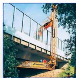
The smallest unit ABC 60 of the range, being mounted on a truck-chassis of 3.5 t. GVW only, is specifically designed to enable quick and easy access to the underside of bridges of limited dimensions. Thanks to its high versatility and high performances, matched with its low cost, the ABC 60 is the ideal machine for both local Road Authorities and private Contractors who are taking care of inspection and repair works of small-size bridges belonging to regional and local road networks.
